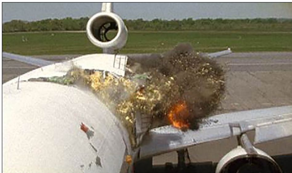
DC-10 jet airliner undergoing vulnerability testing at ATC's Phillips Army Airfield.
