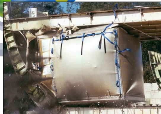
Blast-resistant baggage/cargo container design test in process.
