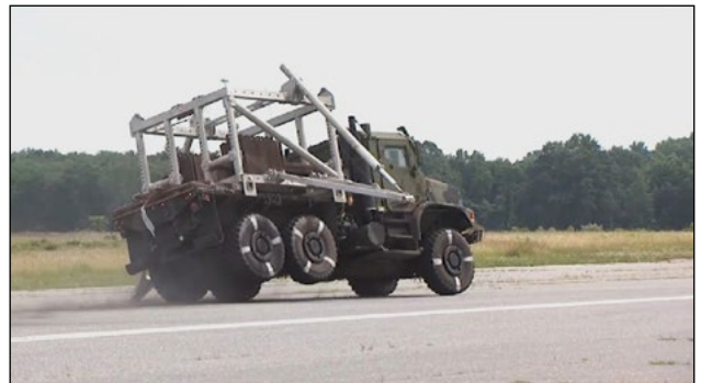
An MTVR with outriggers undergoes a sine-with-dwell test at Phillips Army Airfield.
